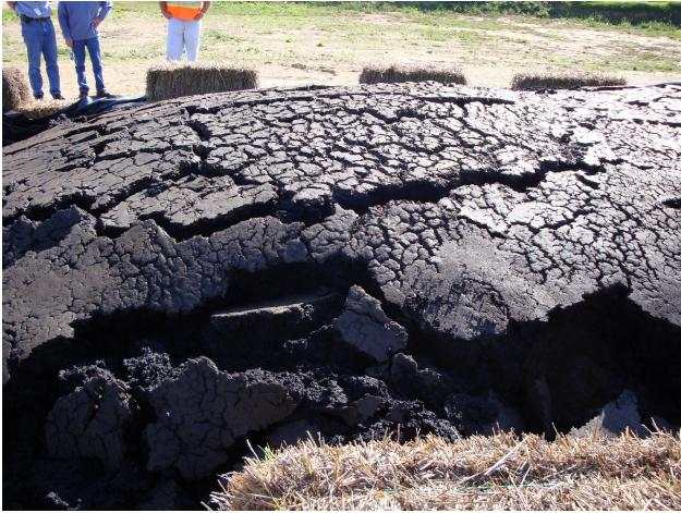
Proper control of the process will result in more and dryer sludge being retained in the bag for disposal resulting in less bag and chemical cost.
