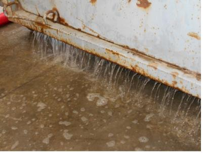
As sludge is pumped into the bag the solids are retained inside the bag. Clear effluent drains out ot the roll off and is returned to the headworks of the plant. When full the roll off is removed to the landfill for disposal.
