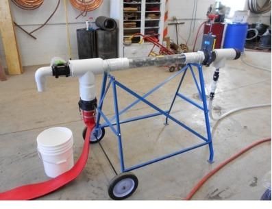
The sludge is pumped from the holding tank to the flocculator where the polymer solution is added. The sludge passes thru the flocculator and solids and water separate and then it is pumped into the bag for dewatering.
