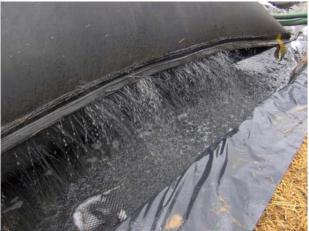
This bag was opened approx 2 weeks after the last pumping. The sludge shown is a municipal waste water sludge. The flocculation process was very well controlled, maximum dewatering allowed these solids to be handled very quickly. Results may vary depending on how well the material is flocked and the process controlled. Most bags are left to dewater for periods of from 2 months to 12 months depending on available space and time.
