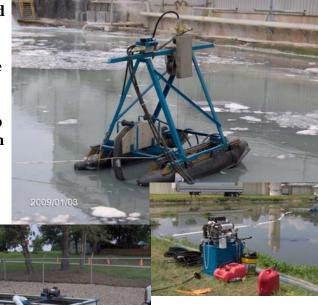
This 24 hp hydraulic unit is used to power the submersible pump on the pumping raft.
