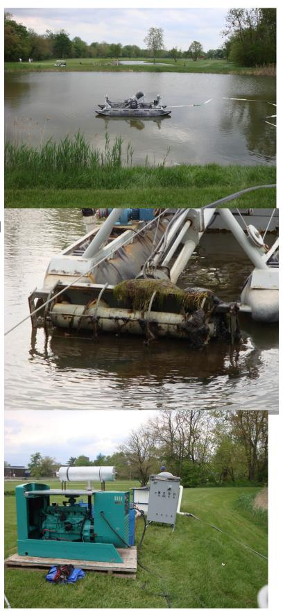
Pumping to a tank on the bank with agitation or recirculation sends a more homogenious solution to the process which improves flocculation.
