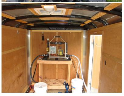
The flocculator causes the water and solids to separate agglomerating the solids so the water can flow easily from the containment bag without blinding.
