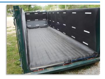
With the right flocculant and equipment, the effluent that flows from the roll off will be clean and free of solids. It will be necessary to return this effluent to the head works of the plant.
