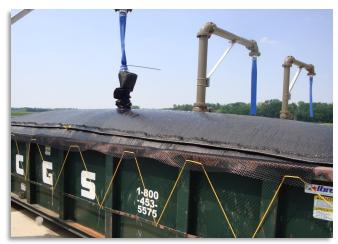
When full, the Blue River Technologies 20/30 yd container bag will hold 15 tons of dewatered solids. The solids will pass paint filter tests and can be disposed of at an approved landfill.
