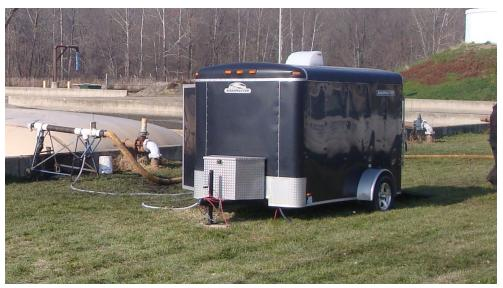
A flocculator on a stand is used to flock the sludge prior to pumping it into the bag. Polymer is pumped from the trailer over to the flocculator, injected into the sludge flow and mixed with the sludge by the Blue River Technologies in line flocculator.
