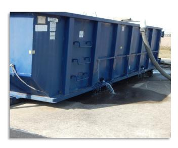
With the right flocculant and equipment, the effluent that flows from the roll off will be clean and free of solids. It will be necessary to return this effluent to the head works of the plant.
