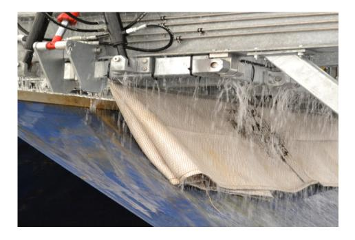
After the three fill and drain cycles, the system will shut down and the operator can allow the batch to drain for any period desired. Typically, the system will be allowed to drain for 6-8 hours before the doors are opened and the load dumped out. Near belt-press quality can be achieved with little to no energy required.
