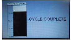
At the end of the drain period, the operator will put the system into manual, open the doors and drop out the solids. Then, another batch can be dewatered.
